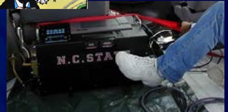
The OEM2100: first-ever mass-produced, commercially available portable emissions device.
